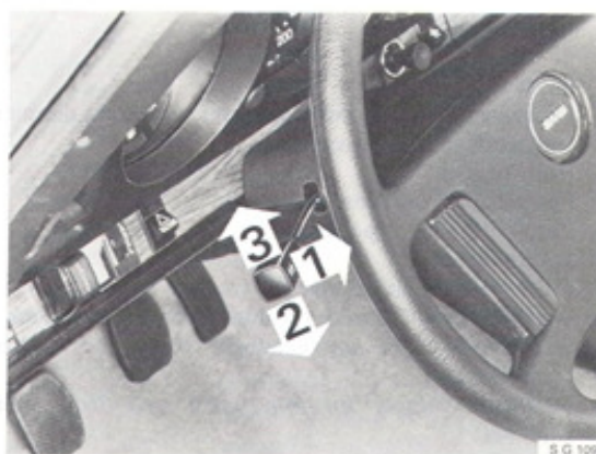
Direction indicator, headlight flasher and dimmer switch
