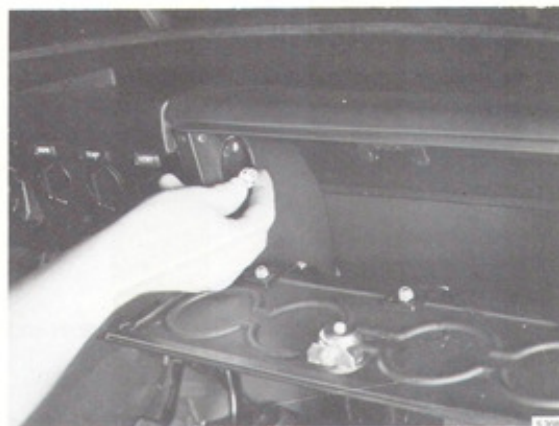
Changing the heater control light bulb
