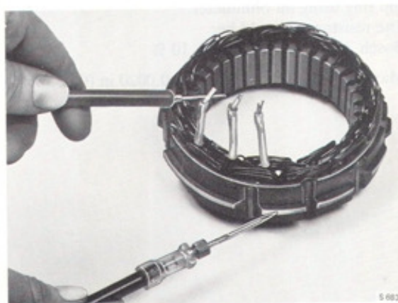
Test stator insulation
