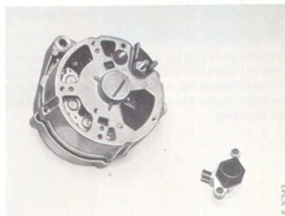
The voltage regulator removed from the alternator
