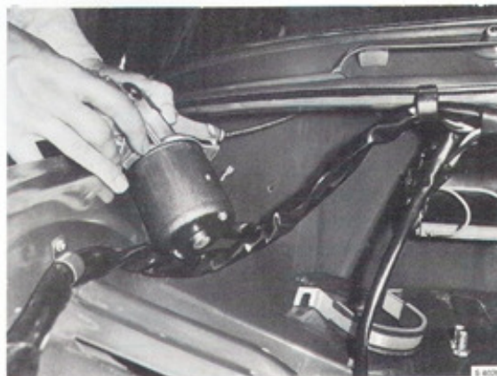
Removal of wiper motor and flexible cable.
