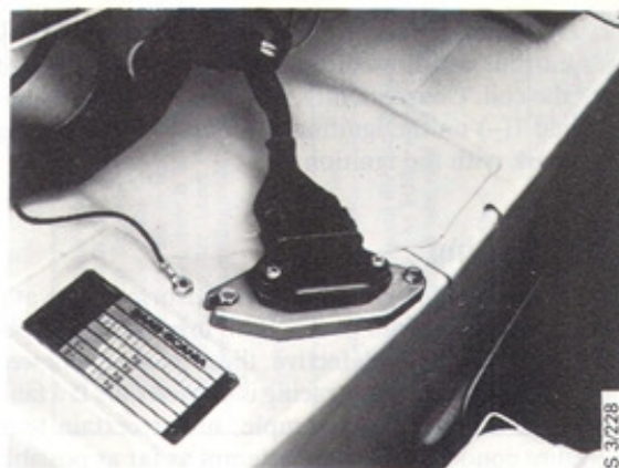
Distributor with Hall transmitter
