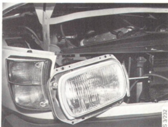
Removing the headlight
