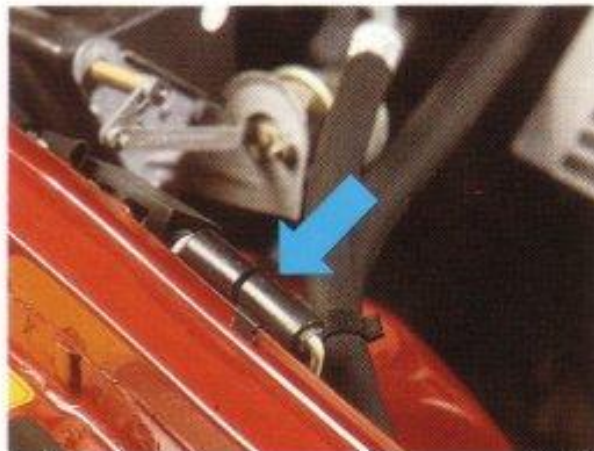
Fuse (25 A) for power supply to pump for Convertible top
