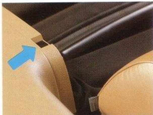
Fastener for middle panel stud
