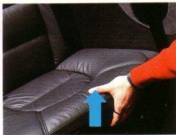
Removing the seat cushion
