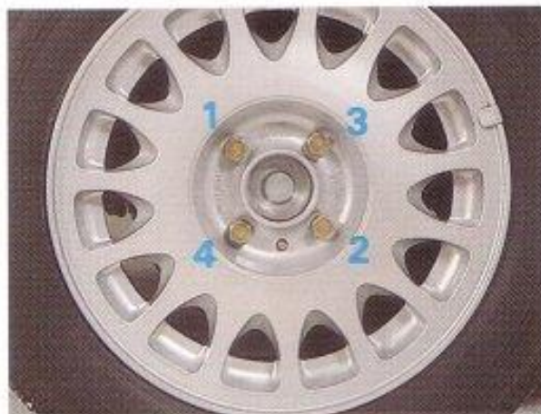
Tightening sequence for wheel studs SG 442
