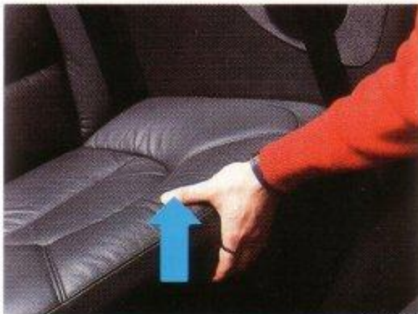
Removing the seat cushion (Convertible)
