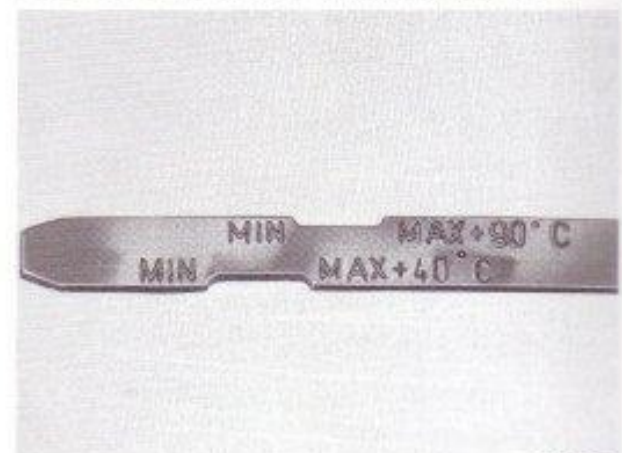
Fluid level dipstick for automatic gearbox
