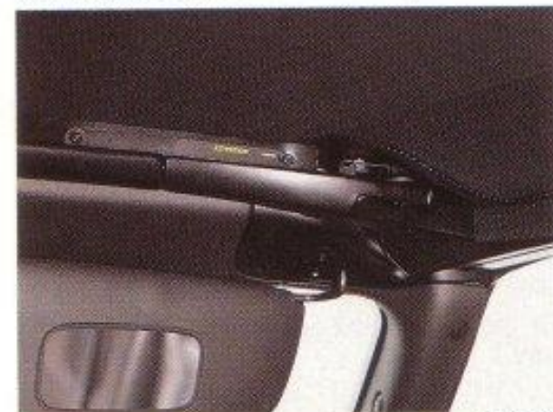
Latching mechanism in locked position
