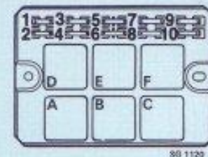
Power distribution panel on LH engine, located underneath rear seat
