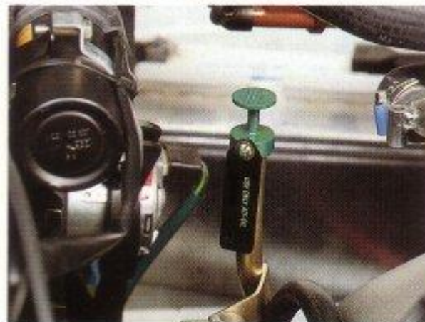
Automatic transmission fluid dipstick
