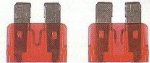
Sound fuse / Blown fuse
