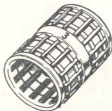
Marking of needle bearings.
