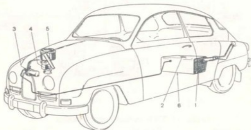
Fuel system Saab 96 and GT 750
