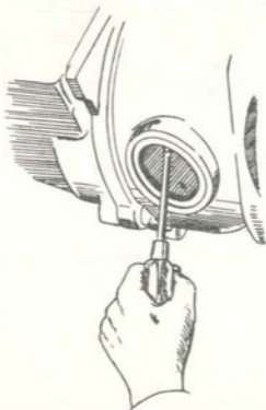
Removal of sealing ring around output shaft
