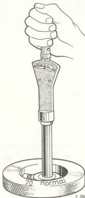
Zeroing the checking gauge
